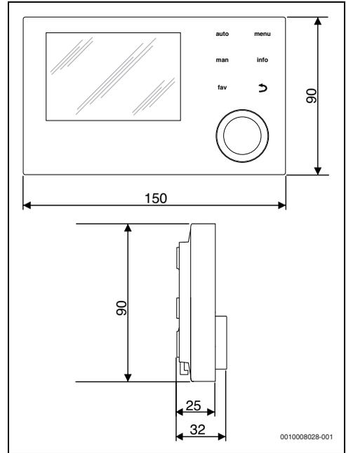
Fig. 4 Dimensioni in mm
